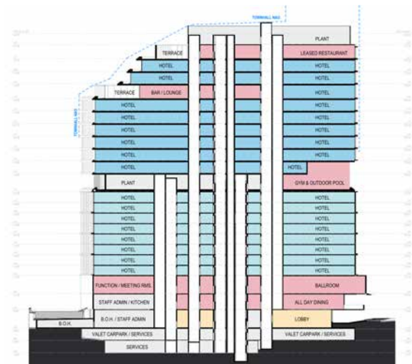
Figure 1: Proposed Building Cross-Section
