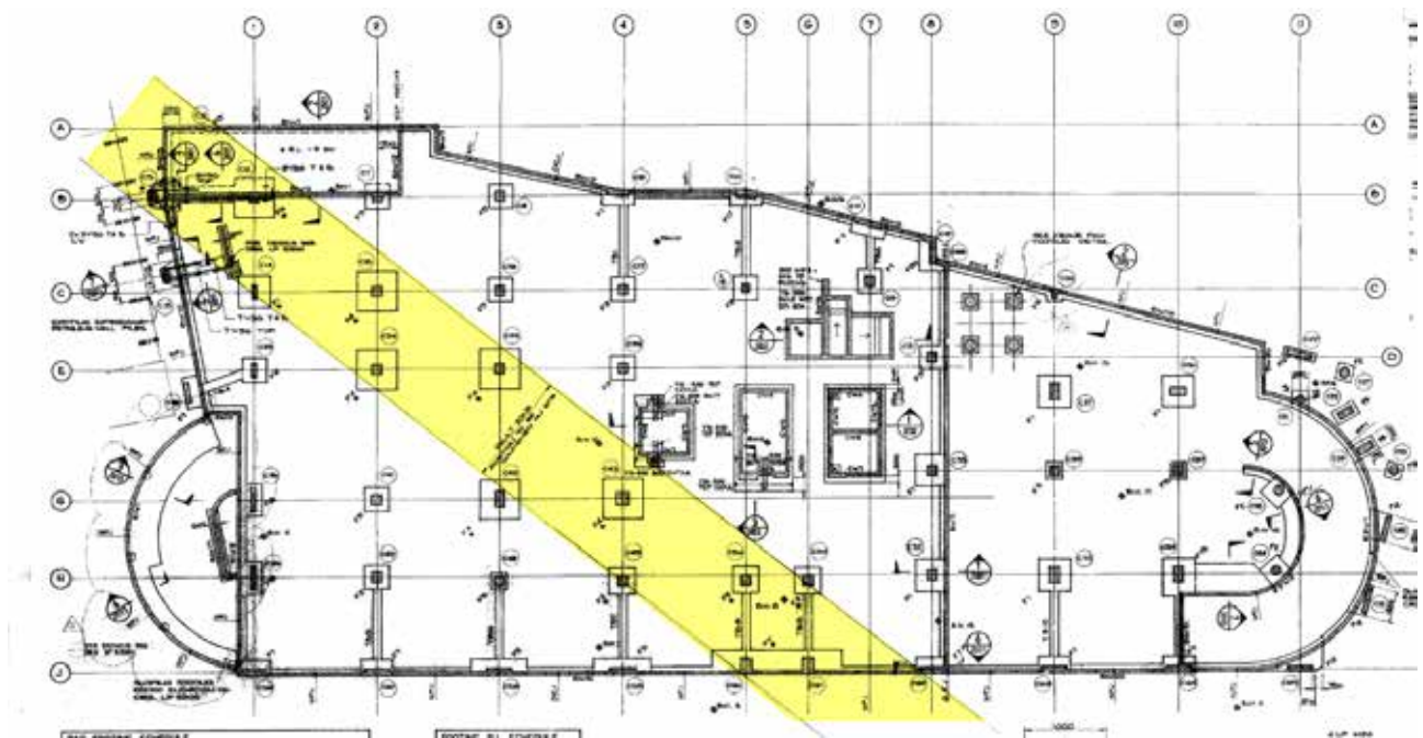
Figure 3: Existing Foundation Plan Showing Fault Zone
