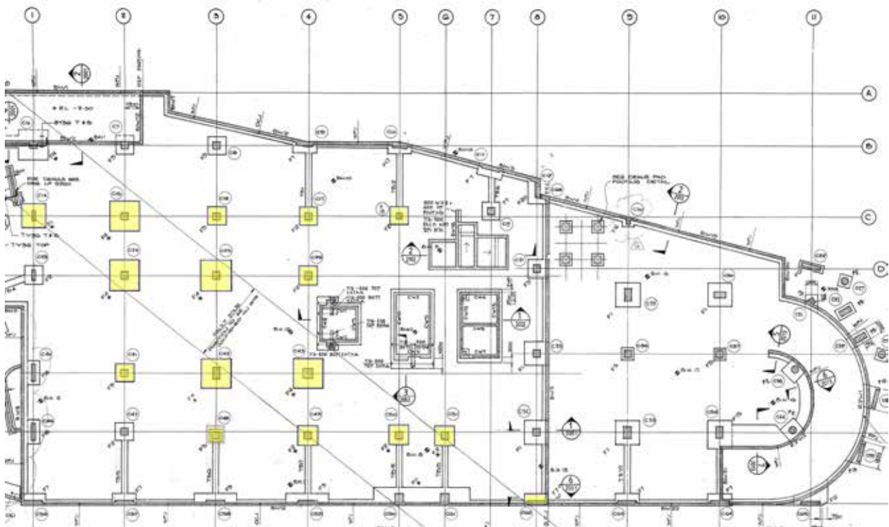
Figure 7: Extent of Foundation Strengthening required
